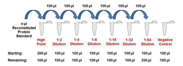
For samples of unknown protein concentrations, serial dilute the experimental sample using Sample Diluent to determine range of detection and acceptable dilutions. Shown below is a diagram illustrating a 10-fold serial dilution on a given Sample of Interest.
