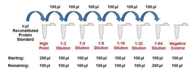
For samples of unknown protein concentrations, serial dilute the experimental sample using Assay Diluent to determine range of detection and acceptable dilutions. Shown below is a diagram illustrating a 10-fold serial dilution on a given Sample of Interest.
